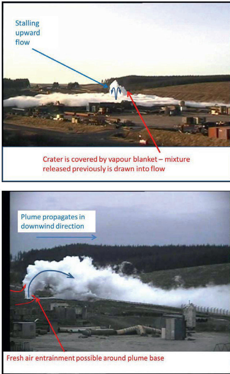
Figure 6. Plume dispersion behaviour – entrainment and dispersion and blanketing
